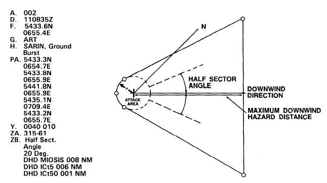
Figure 3-26. Downwind Hazard Area, Type "A" Attack, Wind Speed 10 kts or more.
